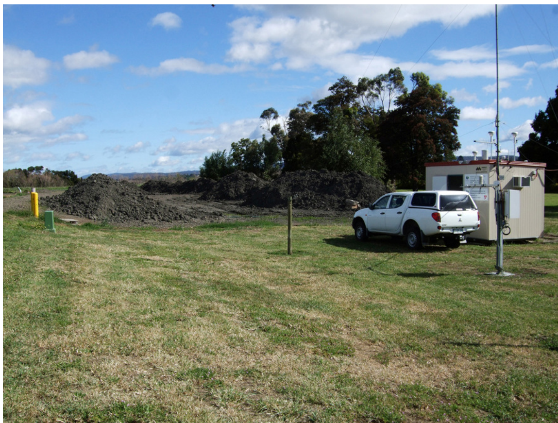
Figure 5. Ti Tree Bend air station (container at right) at its original location (pre-16 December 2008), showing the proximity of (temporary) dirt piles, removed from the nearby settling ponds. In dry windy weather, or when plant vehicles were working here, the air station could experience significant local dust contamination.
